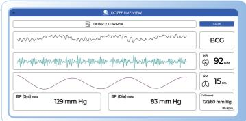
Dozee enables continuous contactless remote monitoring of users with its Al-based Ballistocardiography (BCG) microvibrations and piezo-electric sensors on a chair to extract vitals
